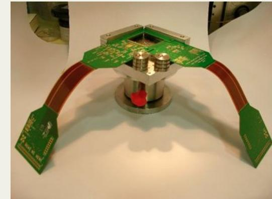
CNM-Barcelona/Detector workbench developed for double side bonding
