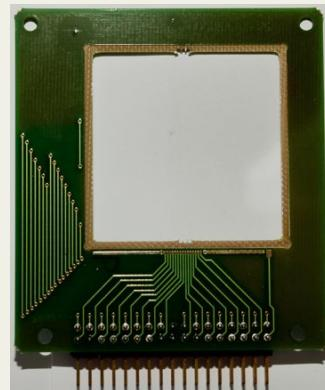
PCB for packaging a DSSSD detector sample
