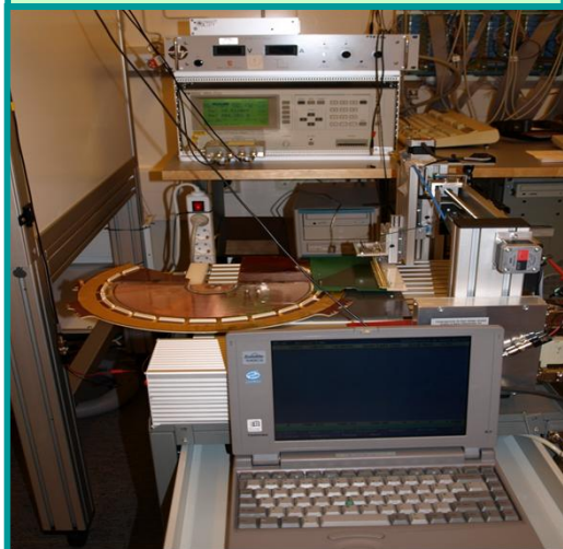
Readout Board Capacitance Distribution Connector 128 strips
