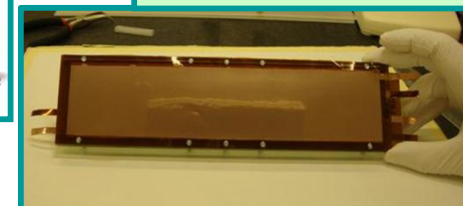
First GEM-TPC called HB1 detector (Helsinki Bratislava prototype 1)
