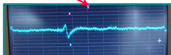
Trigger Signal with rise and decay time reshaped
