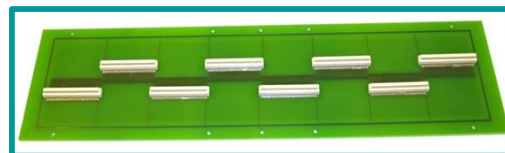
And 8 Header Panasonic connectors with 130 Pin each
