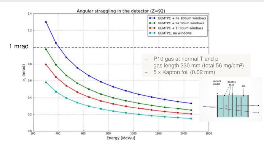
The use of thin & low Z windows to minimize angular spread
