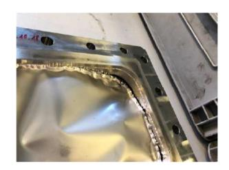
According to in-house experts the right procedure to weld a Ti foil on a Ti frame, is the e-beam technique. A rounded or elliptical shape of the foil should be preferred.
