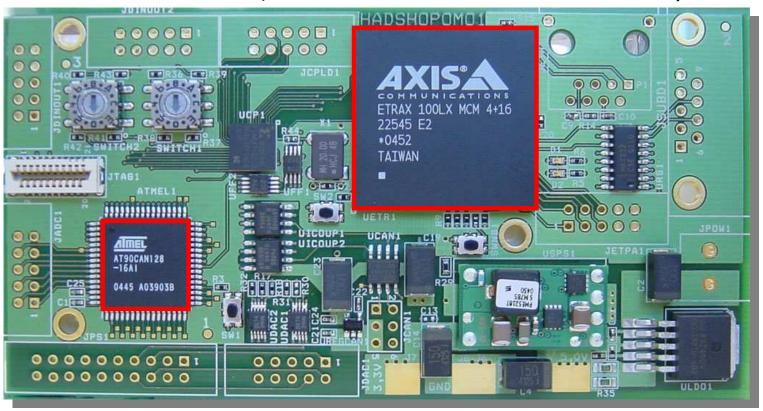
"Multi-purpose control/monitor device developed for HADES [...] is based on the ETRAX 100LX MCM4+16 and runs the "Experimental Physics and Industrial Control System, EPICS".
