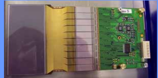
Front of the SSD (thickness 300 \mu m)
