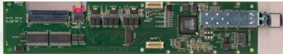
GTB & Piggy back for coupling of 'other' FEEs FE data transfer (Cu/LWL) and Processing
